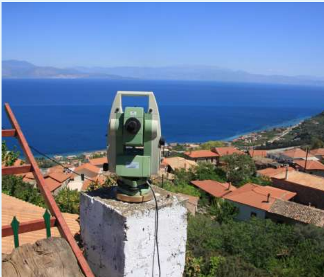
Fig. 10 : Monitoring by Automatic Total Station (ATS)
