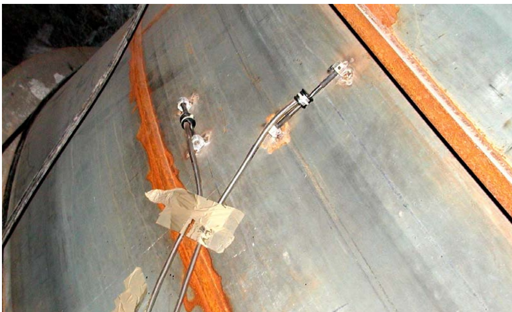
Photo 2. Encardio-rite EDS 20AW strain gages welded on the penstock
