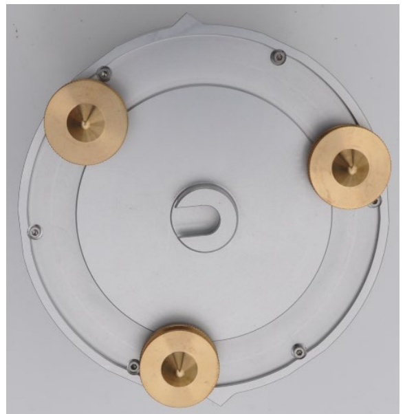
Figure 2 Accelerometer base with fixing point and Orientation indicators machined to the base of the sensor
